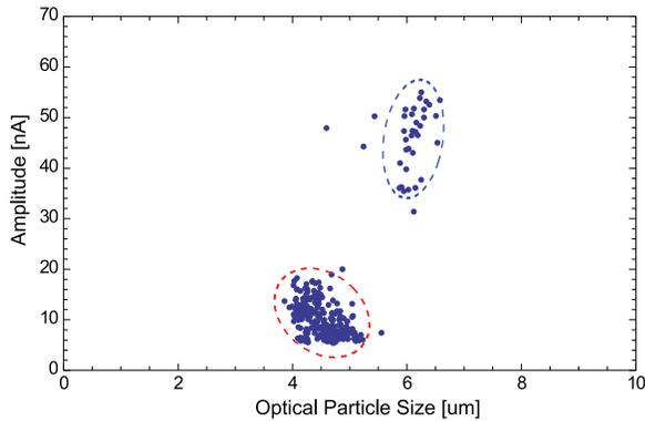
Figure 7: Comparison of the differential impedance measurements (y-axis) to optically measured particle sizes (x-axis). The impedance data were measured at 1.5 MHz.
