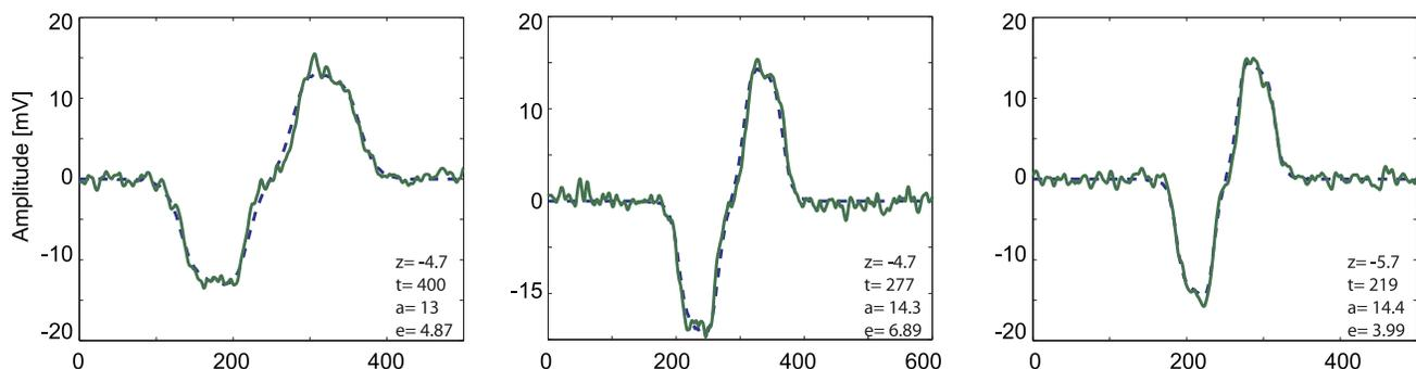
Figure 6: Three examples of transient signals of  $4\text{-}\mu\text{m}$  polystyrene beads passing the measurement area. The solid line is the measured signal, and the dashed line is a template fitted to the measured data. The fitting parameters include amplitude, 'a', vertical offset, 'z', given in  $\mu\text{m}$  with respect to the center of the channel, and time stretch, 't', which relates to the speed of the cell. 'e' denotes the fitting error.
