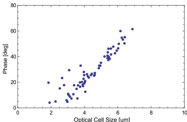
Figure 8: Optical versus impedance measurement data of yeast cells.
