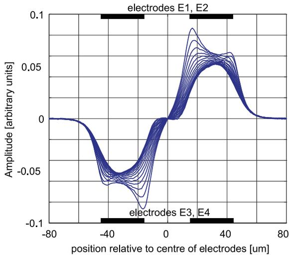
Figure 5: Signals induced by cell trajectories at different vertical levels ( $-8 \mu\text{m}$  to  $8 \mu\text{m}$  displaced from center) as calculated by finite element simulations. The x-axis is the position of the particle relative to the center of the electrodes; the y-axis is the measured signal amplitude change. These signals are used as templates for the measurement data.
