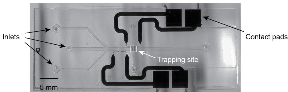
Figure 2: Microfluidic device with three fluidic inlets located on the left side. The left electrode pair is used as reference in the differential measurement mode. The trap for microtissues is flanked by the second electrode pair (white square, see Figure 3).
