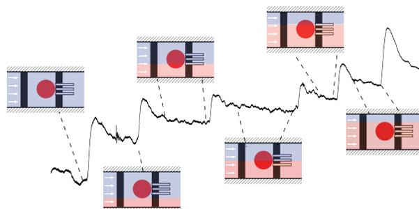
Figure 6: Change of the diff. impedance during a sheath-flow scan across a trapped microtissue (cf. Figure 5).
