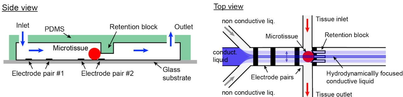
Figure 1: Schematic side and top view of the microfluidic chip. The microtissue is trapped by hanging PDMS blocks in the main channel. Hydrodynamic focusing is used to generate a vertical sheet of conductive liquid that can be scanned across the tissue in order to generate “tissue slices” during the recording.
