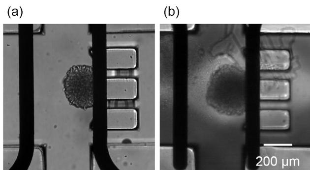
Figure 3: (a) NIH-3T3 brain tumor microtissue containing ~2000 cells trapped in the microfluidic device. The two flanking electrodes are visible. (b) Picture of the channel-centered focusing sheet. Colored liquids have been used for better visibility.
