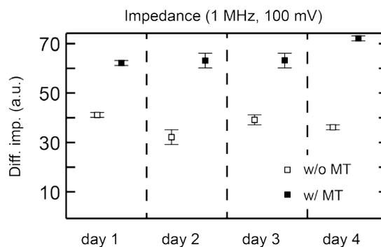
Figure 4: Impedance values with and without MT at different days: a significant difference is reproducibly measured.
