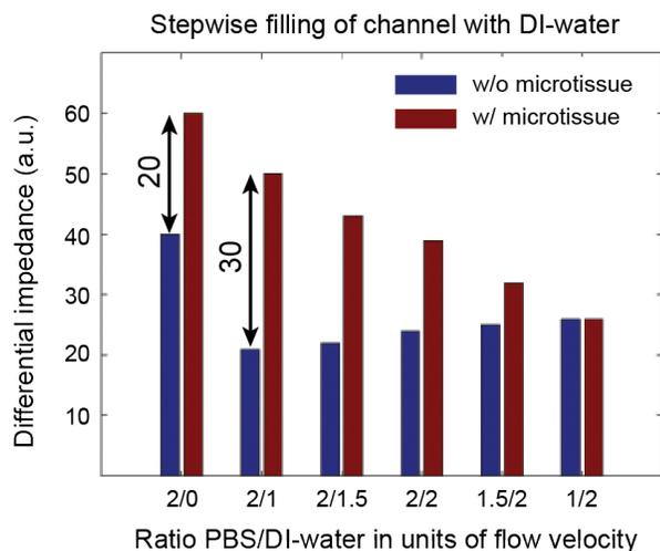
Figure 5: Impedance values during scanning across a trapped microtissue. DI-water is used as non-conductive liquid, the flow-rate of which is continuously increased (see Figure 6 for raw data). Focusing yields a higher impedance difference (=30) compared without (=20).
