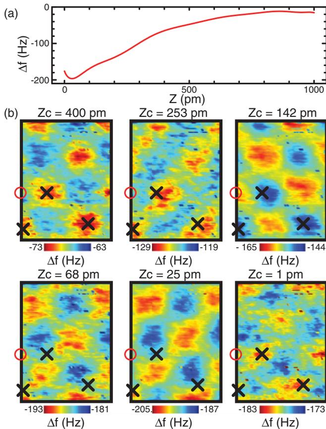
FIG. 4. (Color online) (a) Reconstructed 1D- $\Delta f$  vs. distance curve at a particular site. (b) Constant height images of  $\Delta f$  extracted from the reconstructed 3D- $\Delta f$  dataset at different  $Z_c$ . The location of (a) is indicated by circles in (b). The cross markers indicate reference points.
