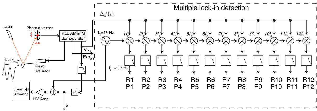
FIG. 2. (Color online) Schematic diagram of the measurement setup based on the multiple lock-in technique.
