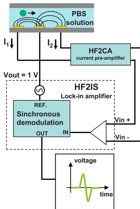
Fig. 3. The principle of differential particle detection based on impedance. Particles flow from left to right in the microchannel and over the electrodes giving rise to a characteristic differential signal.
