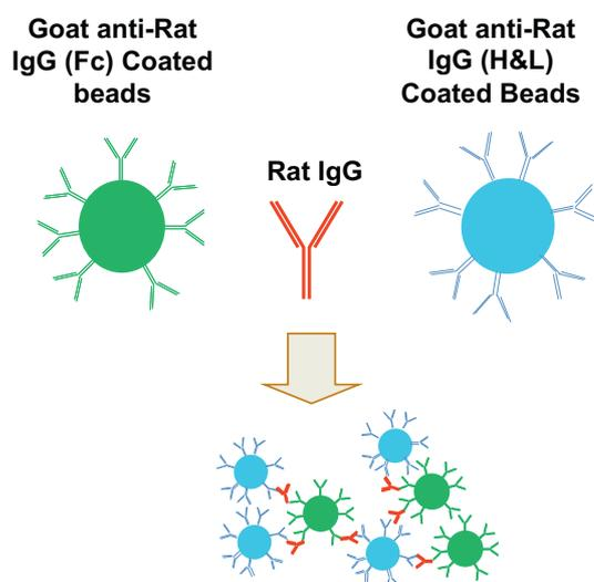
**Fig. 2.** Diagram of the bead oligomers formation. Mixing two sets of anti-rat coated polystyrene microbeads together with rat IgG (target protein) triggers the formation of bead clusters driven by the antibody-antigen affinity.
