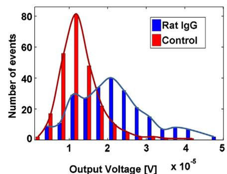
**Fig. 5.** Histograms of the maximum impedance peaks of electrical transitions of rat IgG sample dilution (blue bars) and a negative control (red bars). The means of the distributions are 21.8  $\mu\text{V}$  and 12.6  $\mu\text{V}$  respectively.
