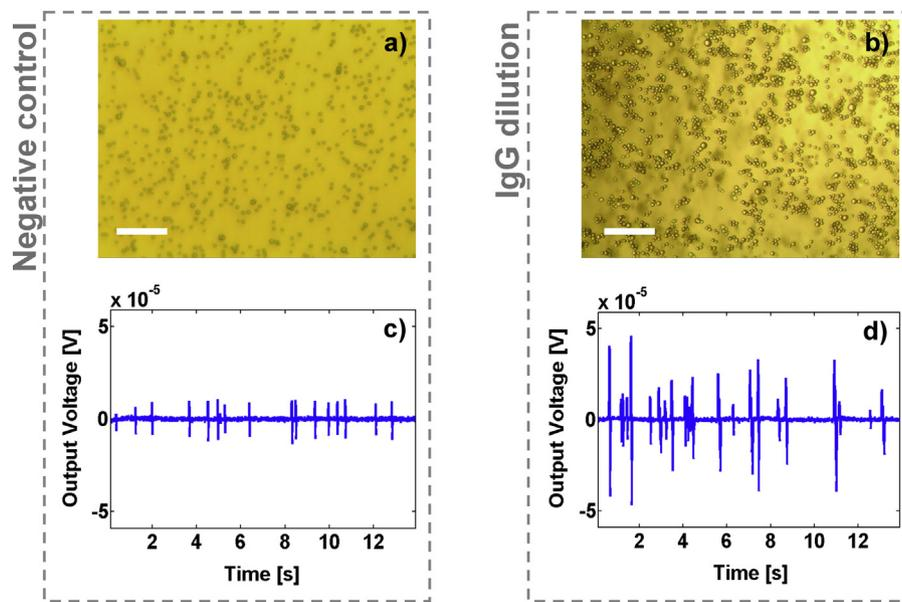
**Fig. 4.** Sample imaging and detection signals. When the protein is not present in the sample (Negative control), little or no cluster formation is observed in the sample (a). However, when the protein is added (IgG dilution), much more clusters are visibly distinguished (b). This condition is also clearly distinguished through the electronic transition peaks obtained for the negative control (c) and the protein dilution sample (d). Scale bars = 100  $\mu\text{m}$ .
