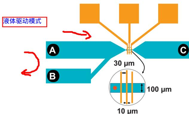
**Fig. 1.** Schematic of the design of the protein detection chamber. The sample is injected through inlet A to fill the volume between inlet A and outlet B. Outlet B is then closed, and a positive pressure is applied at inlet A pushing the sample through the narrow channel where the measurements take place. (For interpretation of the references to color in this figure legend, the reader is referred to the web version of the article.)
